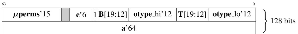
Figure 4.4: Sealed CHERI-128 memory representation of a capability
