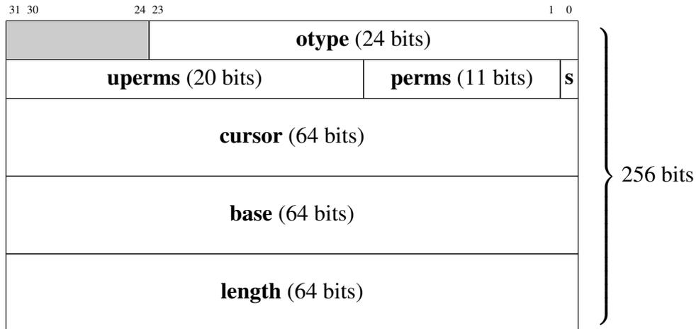
Figure 4.2: 256-bit memory representation of a capability
